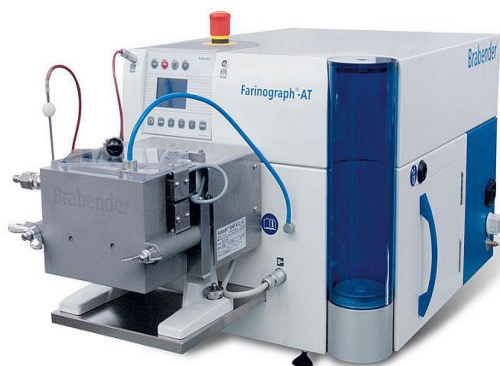
Fig 12: a laboratory equipment to measure the water absorption of flours and determine the rheological properties of the dough
