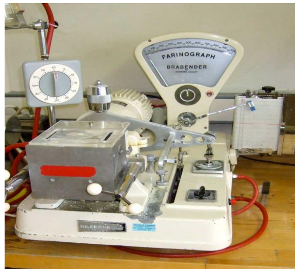
Fig 12: a laboratory equipment to measure the water absorption of flours and determine the rheological properties of the dough
